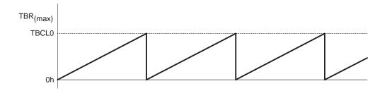
The TBCCR0 CCIFG interrupt flag is set when the timer *counts* to the TBCL0 value. The TBIFG interrupt flag is set when the timer *counts* from TBCL0 to zero. Figure 11–3 shows the flag set cycle.
